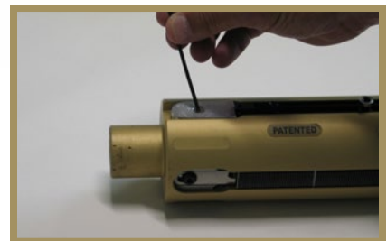
Move the pre-set core positioner track into place and lock. Load up cores and go!
