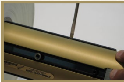
Each contact element moves up and down freely.
