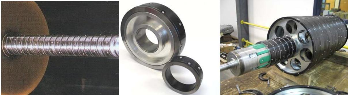
(Goldenrod Model 1250 CL) A cam lock ring grips and locks the inside diameter of the core. The inside diameter of the cam lock ring then becomes the point of friction on the internal pneumatic shaft. The cam lock rings rotate on the internal pneumatic shaft which utilizes engineered materials (high temperature plastic or felt over a bladder system) to expand and control the amount of slip.
