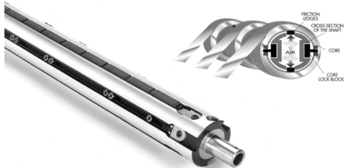
Core clutch shafts (Goldenrod Models 1250 DFX & DFB) create torque proportional to core width. Friction ledges are controlled pneumatically and contact the cores inner diameter. Wider cores engage more frictional elements and receive more torque than narrow cores. Heat, dust and torque variations are much improved over the older “Yoke” system.
