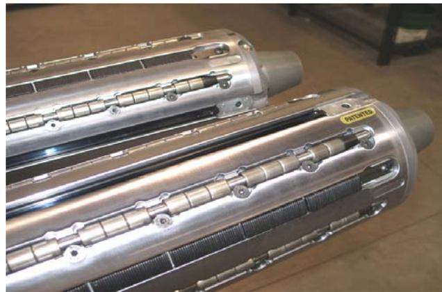
**OPTION 4** – Upgrading from a YOKE system that does have a separate rewind drive system to a Locked Core Internal Clutch Design.....or Goldenrod Model 1250 CL Cam Lock.
