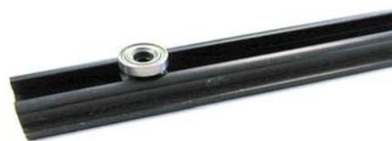
Side-lay Adjustable Core Stop Ledges
