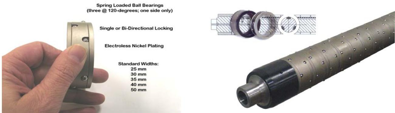
The differential shaft must be driven at a 3 – 10% over speed at all times. All the cam lock rings need to slip continuously. As the roll diameters build, the differential shaft rpm must decrease to maintain the same over speed, and the air pressure usually increases to maintain the same tension. A feedback loop that compares the line speed, roll diameter, and rewind motor speed can be used to control the over speed.
